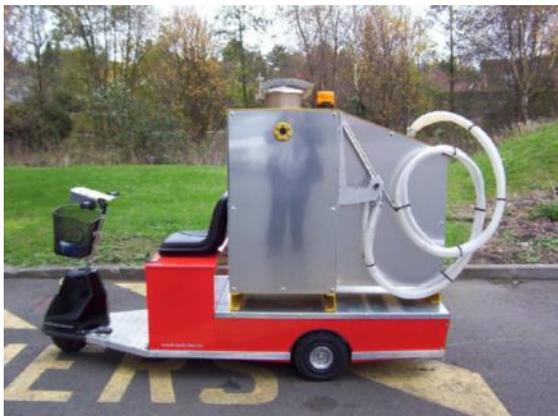
The **NEU MOBISAND LMU Type** is a light mobile unit for sandbox filling, completely self-powered during the sanding operation. Its small size enables a rapid access to hard-to-reach areas. It is particularly suited for filling small sandboxes (sand flow from 10 to 15 l/min) or where occasional filling is needed.
